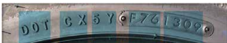
DEPARTMENT OF TRANSPORTATION MANUFACTURER & PLANT CODE TIRE SIZE CODE MANUFACTURER IDENTITY NUMBER WEEK AND YEAR TIRE WAS MADE
