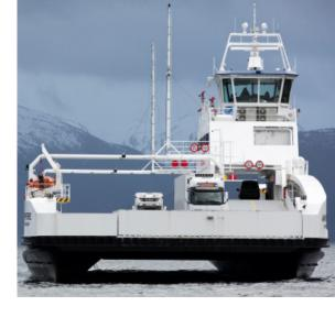
Passengers, crew and residents of the picturesque villages of Lavik and Oppedal at either end of the crossing will appreciate the ferry's emissions-free and near-silent operation. Since the ferry is run entirely on battery power, it does not emit greenhouse gases or particulates. The vessel's batteries are recharged using hydroelectric power from the existing electric utility grid infrastructure in each village, further minimizing the impact of the ferry service.
