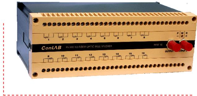
The RFM-16 analog multiplexer converts 16 Pt-100 sensors to temperature linear 12 bit output data.
