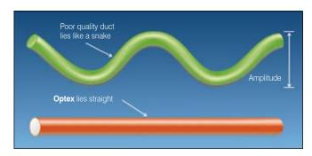
The relationship between the COF and cable tension is not linear, it is exponential. A small reduction in COF can result in a very large reduction in cable tension. See graph on opposite page. This is because all practical duct installations have some amount of bend in them: they are never perfectly straight. The following experiment shows how bends affect cable tension. A cable is pulled into a duct that is still on a drum.
