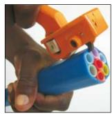
**Bending performance** The minimum bending radius is 10 x outside diameter. For example a 12mm **Microdux** has a minimum bend radius of 120mm, and a 7 way 12/9 protected **Microdux** with an OD of 40mm will have a minimum bend radius of 400mm.
