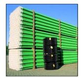
Unpalletised conduit should not be stacked more than 1.8m high. The conduit and couplings are UV stabilised and can be stored outdoors for up to one year.
