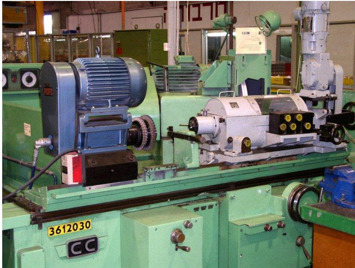
Dedicated Grinder C. C. for Grinding Turbine (High Speed) & Compressor Rotor (Low Speed) Blades
