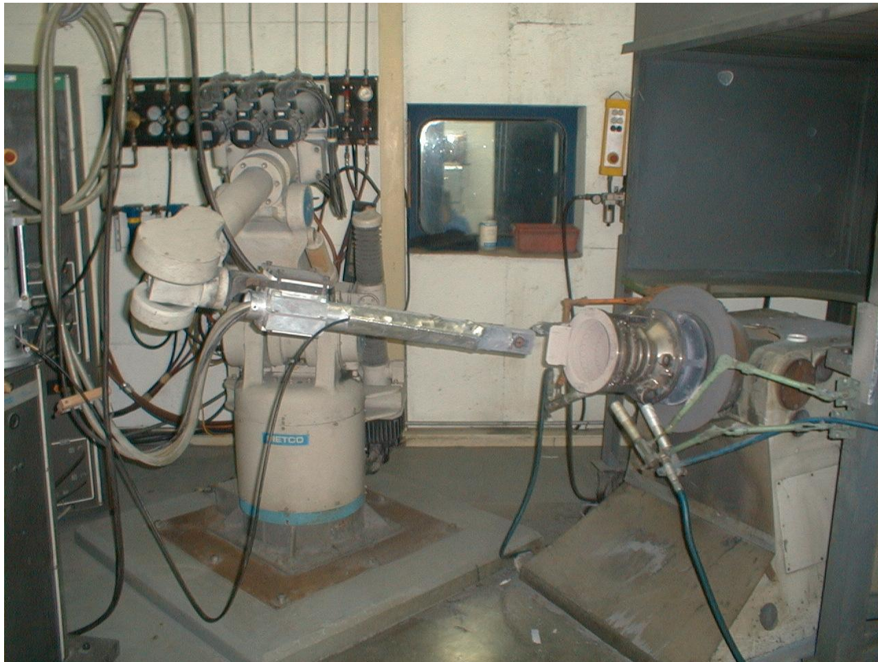
T-700 Compressor Case Flowpath Plasma recoating
