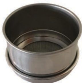
75mm STAINLESS STEEL LABORATORY TEST SIEVES
