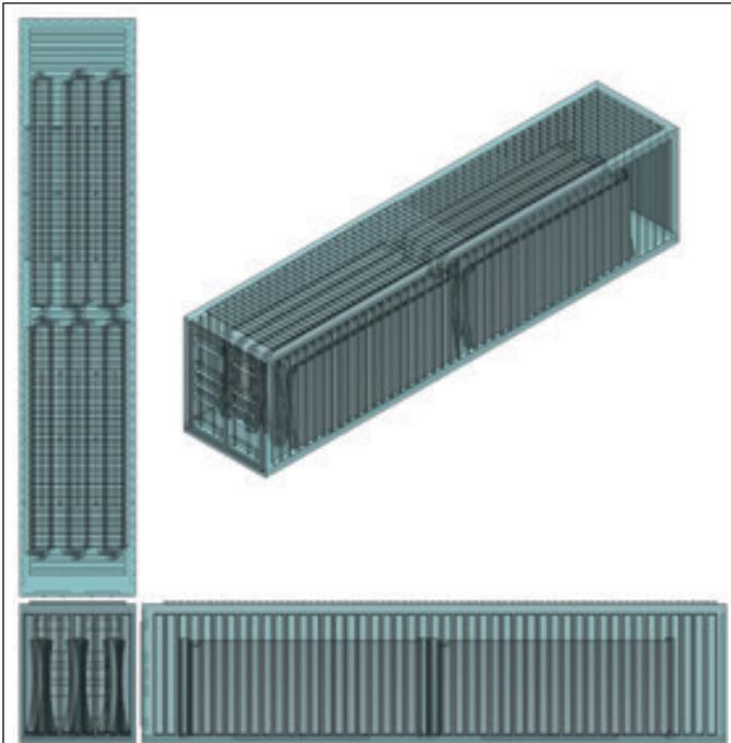
Forty-foot container with 1 W-Tank® Storage Tank consisting of 44 plates Salamanca, H=5m, D=29m and capacity of 3,303 m<sup>3</sup>.
