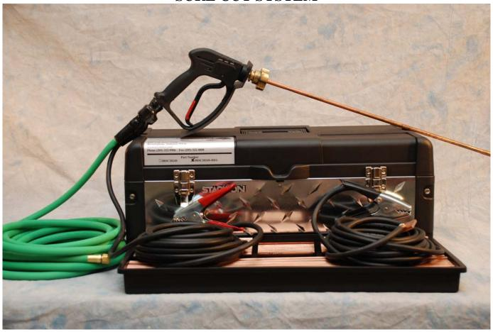
The Oxylance Sure Cut system will cut virtually any metal, both ferrous and non-ferrous, and is faster than conventional oxy-acetylene cutting or carbon arc gouging. The Sure Cut exothermic cutting rods don't require preheating or cleaning of the material prior to cutting. It is easy to use and is cost effective for most applications.
