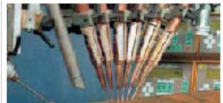
Up to six wires can be used together, each with their own power source. The lead wire is usually DC+ polarity with the trailing wires being AC. Speeds of up to 2.5 m/min can be achieved giving a maximum deposition rate of 90 kg/h. This technique is particularly suitable for longitudinal pipe welding.
