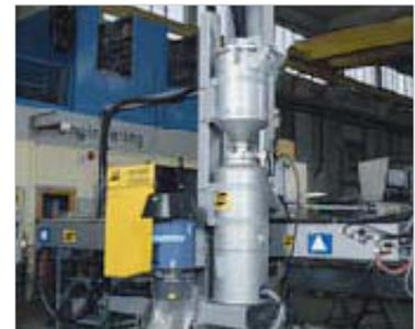
ESAB has different flux equipment/systems to combine with automatic submerged-arc welding equipment. The OPC flux recovery units have a robust, compact design – easy to fit and easy to use. They can be fitted equally well to A2 and A6 equipment, both stationary and travelling. The FFRS-systems (flux feed and recovery) are designed for continuous, high-capacity welding operations. They are ideal for long runs and mass production.
