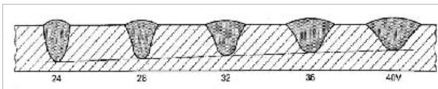
Effect of arc voltage on weld profile.
