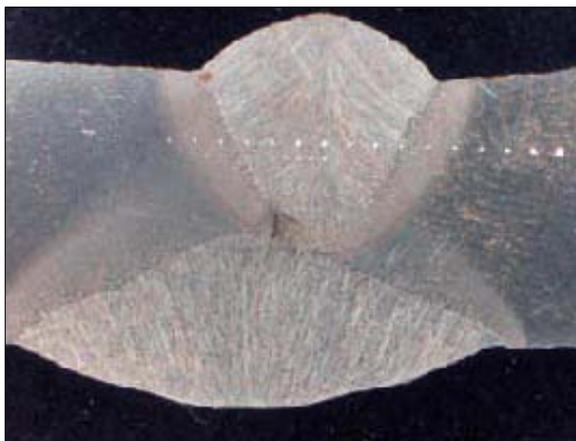
Insufficient penetration and excessive reinforcement; also misaligned.
