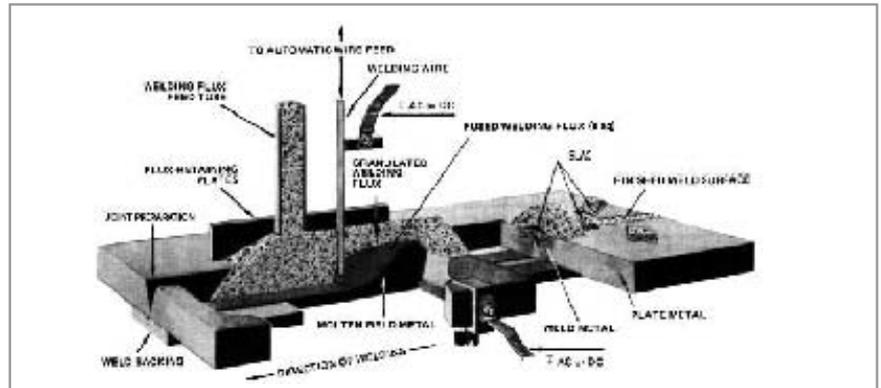
current flows between the electrode and the work.
