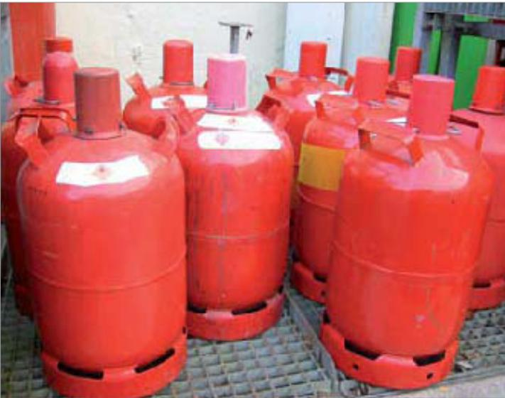
The typical plate thickness for air compression tanks and gas bottles is 2.5mm. The overlap joints are SA welded with 1.2 to 2.5mm diameter wires.
