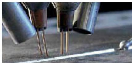
The ESAB tandem-twin process involves two twin wire heads placed in sequence. With the use of 4 x 2.5mm diameter, wires deposition rates of up to 38 kg/h can be achieved. The process can be used in joints that allows accessibility for the equipment, e.g. circumferential welding in wind tower fabrication.
