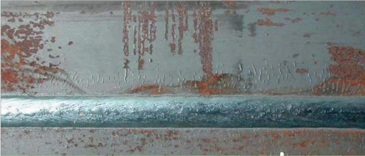
**OK Flux 10.88 on rusty plate with mill scale. Porosity-free, shiny weld appearance. Clean weld with no indication of slag residues adhered onto the bead or along the toes of the weld.**
