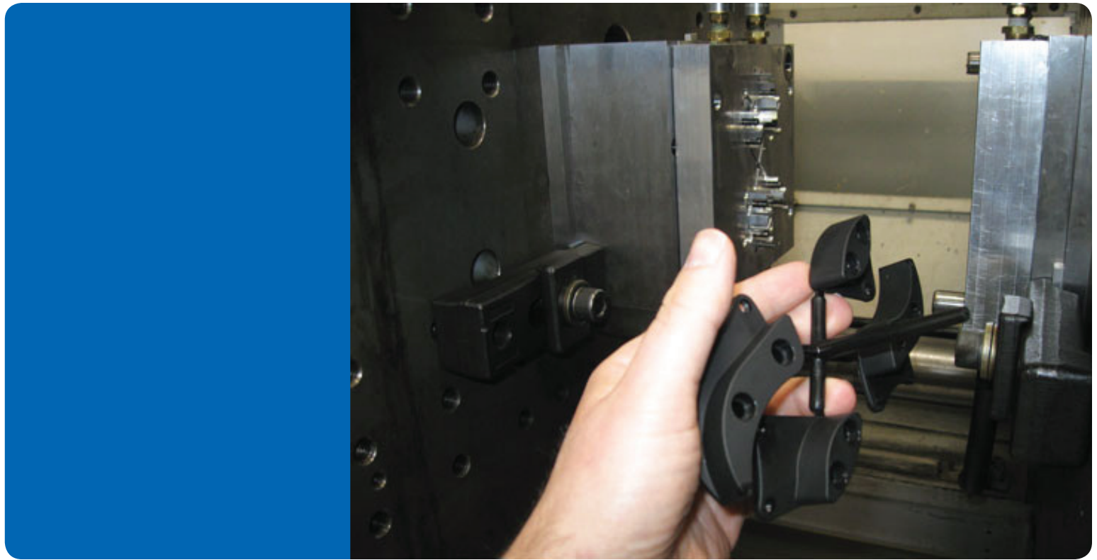
Straitline's machine shop also produces its own plastic parts. This injection-molding press uses molds machined in-house.
