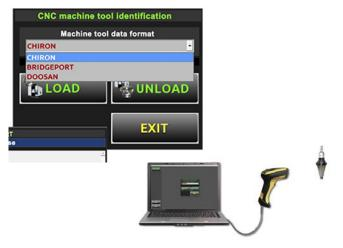
**Step 2)** Remove tool from presetter and bring to the CNC machine. Select the machine model you are loading tool into on your laptop or tablet.
