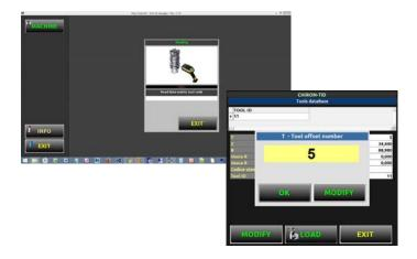
**Step 3)** Once tool data is scanned into the tool database, select tool number you wish to save to in machine tool list.
