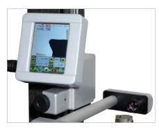
Integrated LCD touchscreen / vision screen for quick and easy operation.
