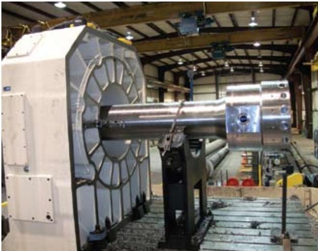
**Features are oriented to two rows of 16 holes—16 tapped and 16 thread-milled holes—in each row along the OD of the part. There is also an API ring groove on a milled flat behind the hub of the OD that is oriented to these OD features and has an intersecting hole from the face of the part.**
