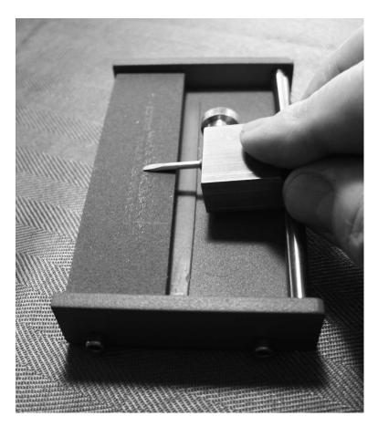
putting the slider on the rail and pressing on the end of the blade against the stone. Then tighten the thumb screw. Holding the slider as shown, run it back and forth until one side is done, and then flip the slider over to finish the other side - assuring both sides of the blade to be parallel. Set the end thickness by rubbing the tip over the stone - while still in the slider - until the desired end thickness is achieved.
